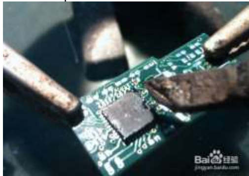
7. Use a soldering iron to tin the pins on the chip side
